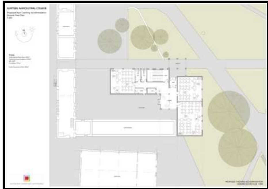
A 2D plan of the internal structure of the proposed building- highlighting the two new 30 seat classrooms, and 60 seat classroom.
